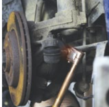
Loosening track rods
