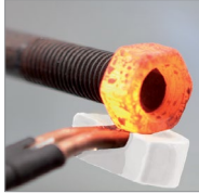
Release rusted bolts
